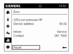
Press the control knob. The text changes to "Confirm" and is displayed inverted
